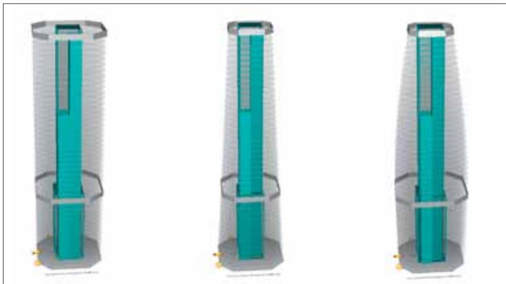
Figure 6 Extruded, Inclined and Bowed Elevations
