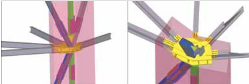
Figure 10 Steel Diagonal/Megacolumn Connection (TEKLA)
