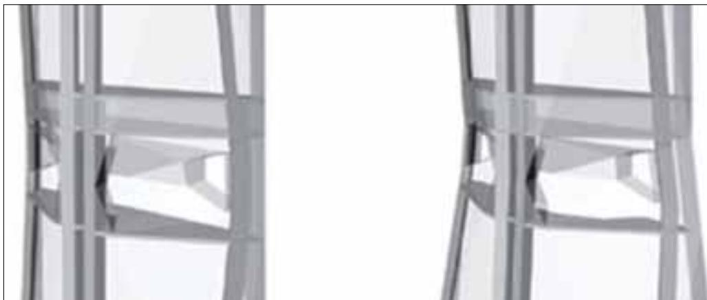
Figure 11 Concrete Megacolumns at Fuselage (Opening) Levels
