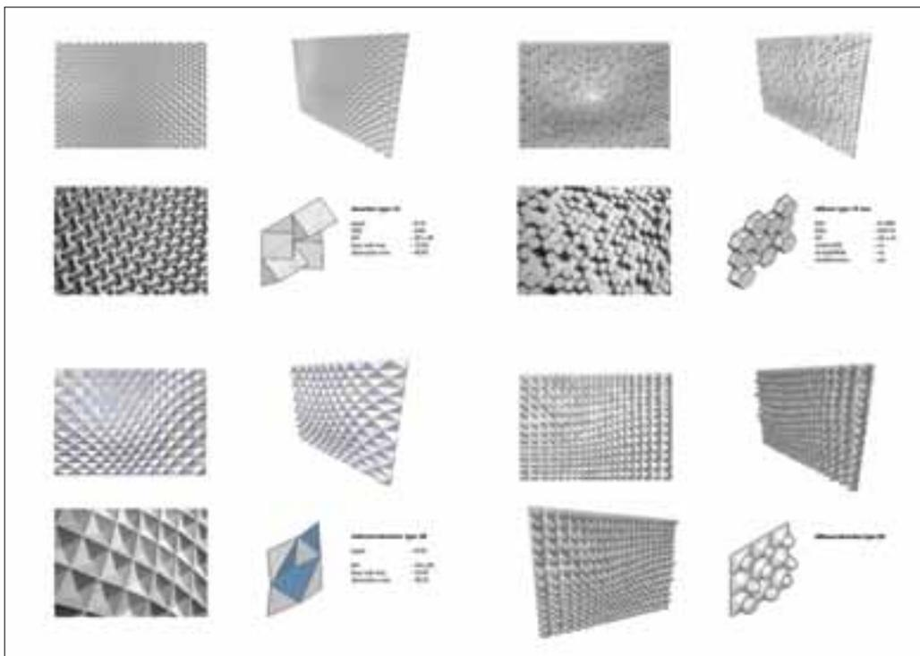
Figure 3 Four acoustically regulating surfaces, clockwise from top left: an absorbing surface, a diffusing surface, a combination diffusing/absorbing surface, and a combination absorbing/reflecting surface
