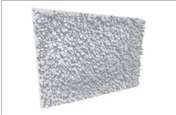
Figure 5 Random radius, random depth circle diffuser based on circle packing algorithm
