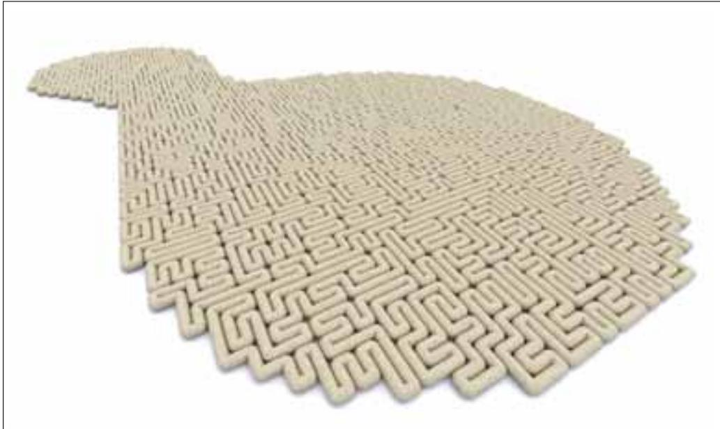
Almost all Rapid Manufacturing processes work on the basis of horizontal slicing; the height generated by this sequential layering is usually called the z-height (hatching and contouring on a given layer occurs in the x and y directions). With a visible building resolution, however, it is easy to imagine how to create tool paths that occur in all three dimensions (fig. 7). With Rapid Prototyping software packages, all the slicing is done purely horizontally, and the G-code follows that concept.
