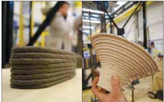
Figure 5 Resolution of Concrete Printing
