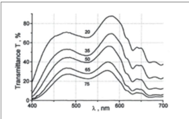
Figure 8 Transmissivity of thermochromic glazing with wavelength and temperature
