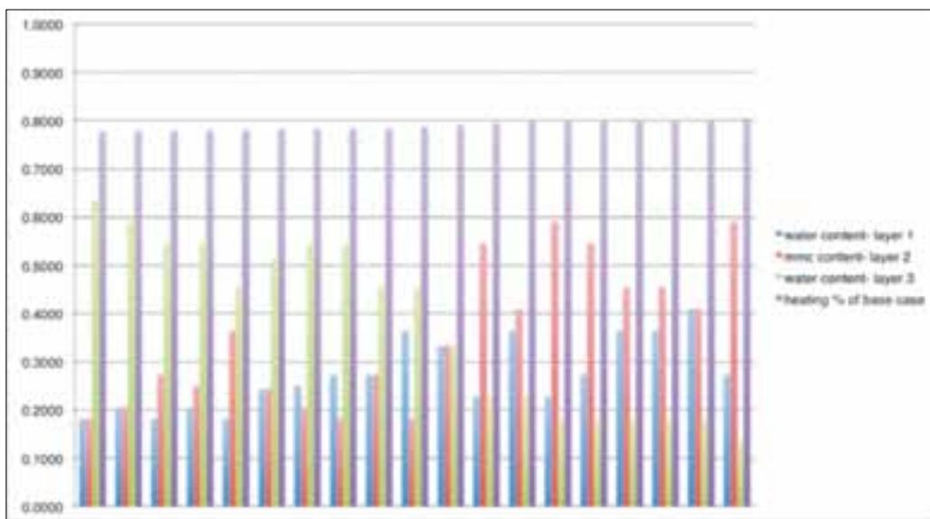
Figure 15 Assessment of heating zone area of a water-mmc-water wall in relation to the distribution of water and mmc: water content in outer layer (blue), mmc content (red), water content in inner layer (green), and heating zone area as a percentage of the base case (purple)
