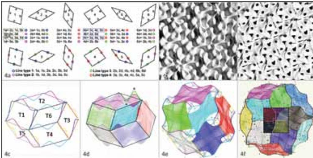
Figure 4: 4a Adjacency analysis from the 4d tiling shown in figure 3b; 4b 5d and 4d NURBS tiling; 4c 6 tiles in 4d showing 4 different line types in sets of 2 for each NURBS tile; 4d Same as 4c with parametric curve line type at edge of tile; 4e. NURBS tiles with openings at the vertices; 4f 5d tiling (10 tiles) with tangential offsets
