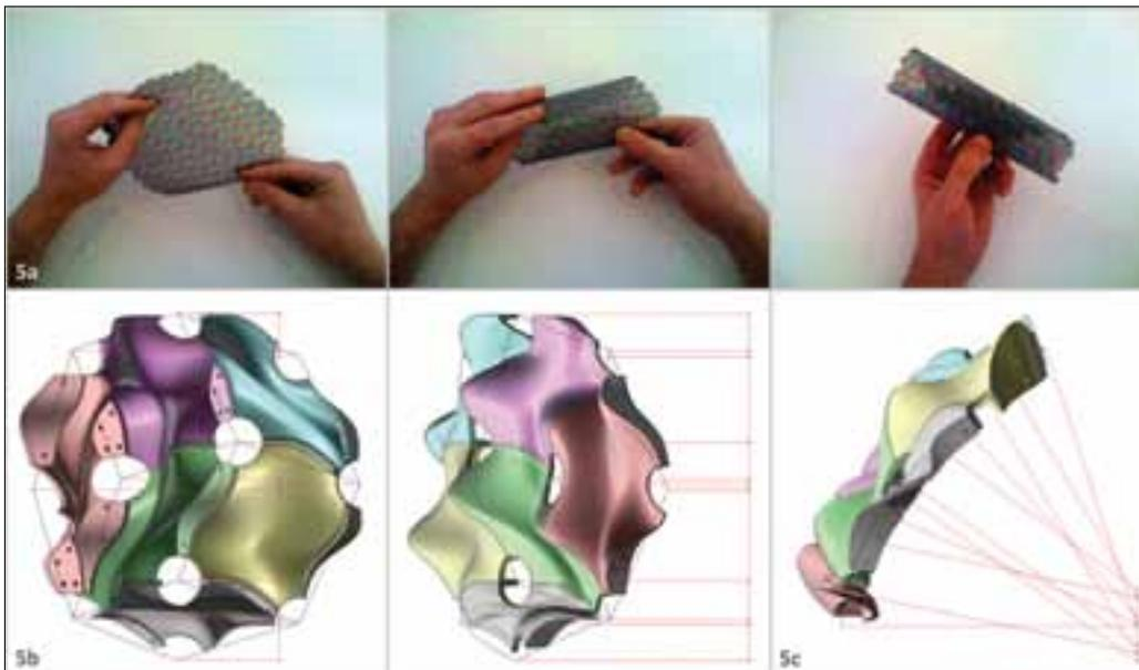
Figure 5: 5a Rolling of a 4d tiling into a cylinder; 5b Views of 6 NURBS tiles with openings; 5c Side view of NURBS tiles converging to the central axis of cylinder
