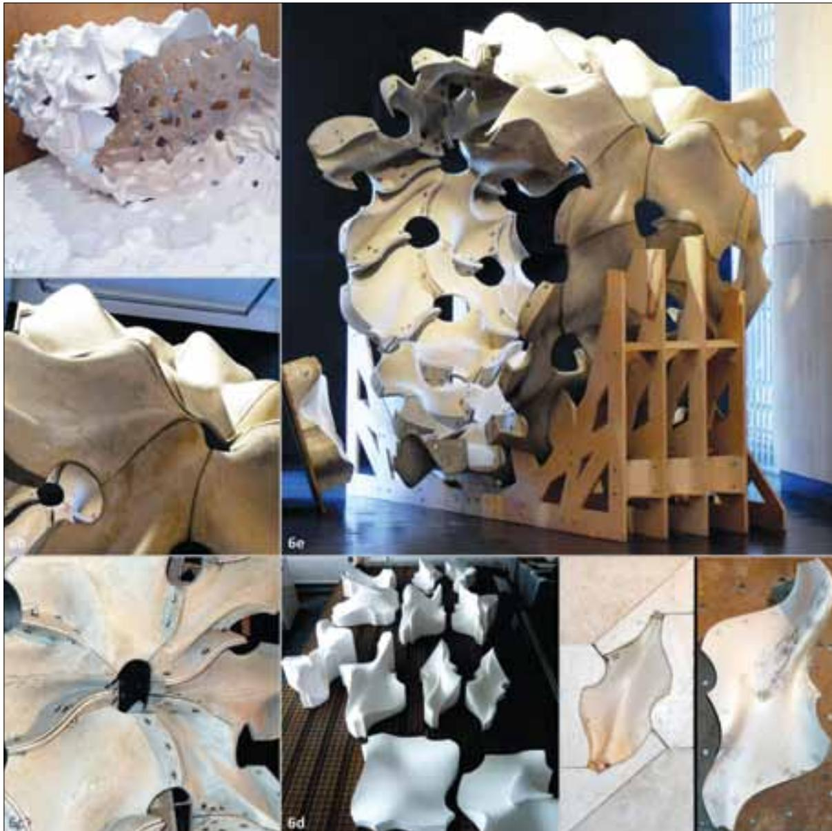
Figure 6: 6a Field model of 4d cylindrical NURBS tiles; 6b Close up of prototype showing exterior flow between elements; 6c Close up of interior assembly; 6d Polystyrene part moulds for concrete casting; 6e Full scale prototype of quasi-roller
