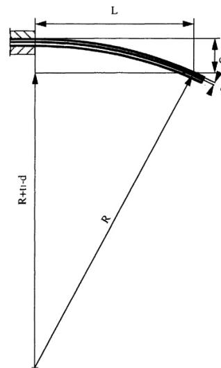
Figure 3. Bending of a bimetallic strip fixed at one end
