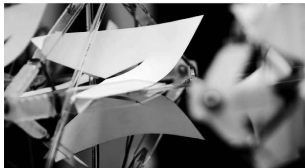
Fig. 7. Prototype 3 with air muscles actuation creating surface contraction
