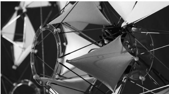
Fig. 3. Prototype 1 with rotational servomotors and actuated discs
