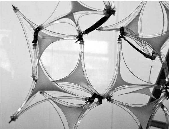
Fig. 9. Prototype 4 with linear cross component air muscles
