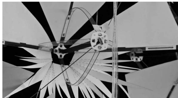
Fig. 5. Prototype 2 with linear actuated air muscles
