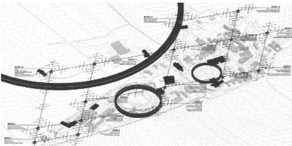
Figure 8. Diagram of the Meyrin Transit-Energy Grid showing existing buildings (blue), existing buildings selected for general upgrades and integration into the proposed grid infrastructure (black), and existing underground particle colliders (black).
