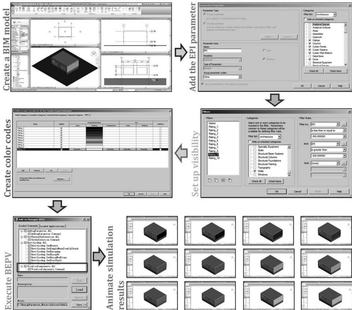
6 Workflow of BEPV using Autodesk Revit and its API
