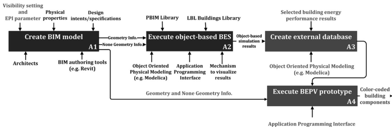
1 Overall process diagram using IDEF0. Dark blue components represent the thermal simulation prototype of our Physical BIM project, and dark red shows the BEPV workflow
