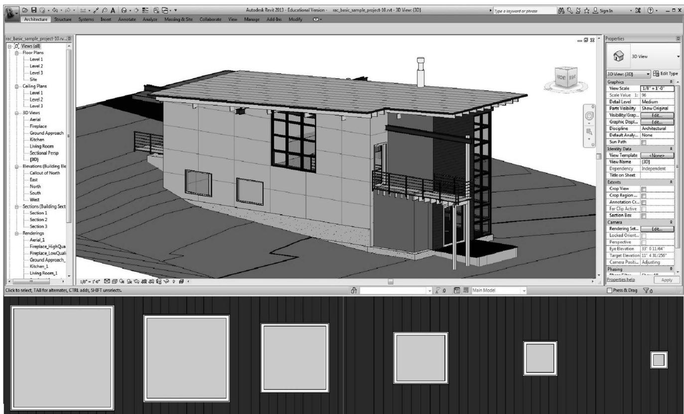
2 The BIM model of the case study with different window sizes that can be parametrically changed by Revit2GBSOpt
