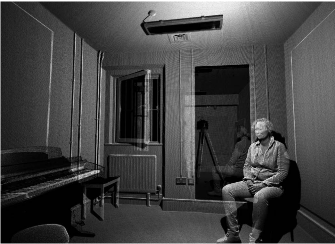
2 The Crying Room. The scanner captures the figures blind side through the rebound of signals from an adjacent mirror.
