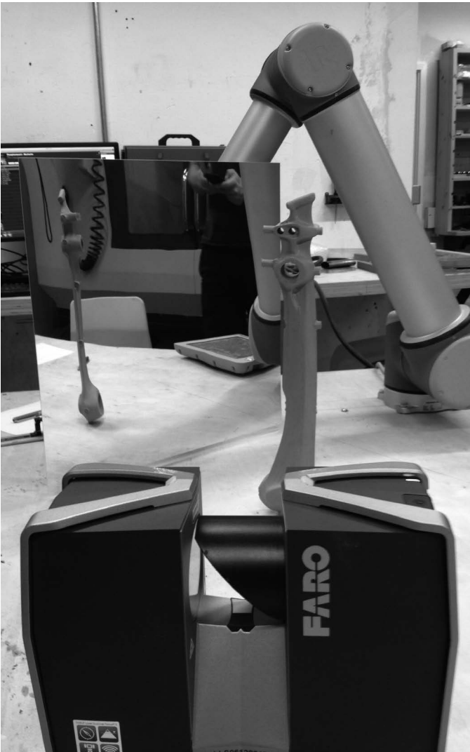
10 Robotic arm is fitted with a reflective panel and sent a command to sweep in an arc whilst the event is scanned.
