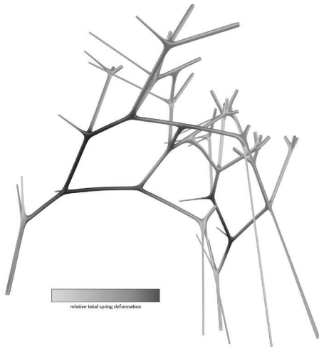
10 Overall generation with registration of absolute stresses derived during formation in the spring-based simulation engine, and local assignment of total material thicknesses according to this registration
