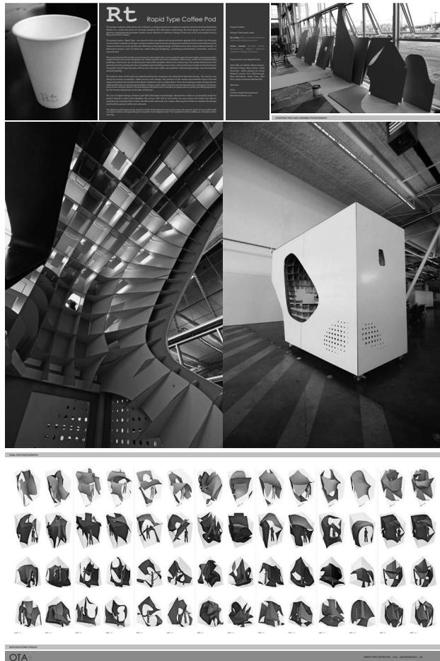
The exterior form of the pod was determined by the maximum size allowed for towing. The interior was driven by human occupation, coffee service, and storage. The studio pursued a design process utilizing Booleans to quickly test multiple schemes while addressing the tension between the orthogonal container and a more complex interior. The final design offered the most variation of space and use, while providing opportunities for human interaction on all sides of the pod.
