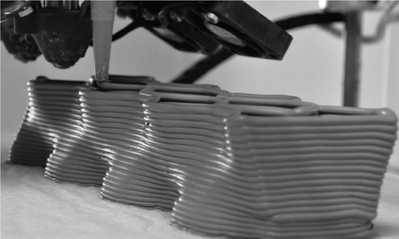
1 Brick being printed on a desktop 3D printer
