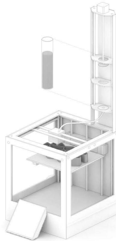
2 Diagram of desktop 3D printer with custom extrusion system
