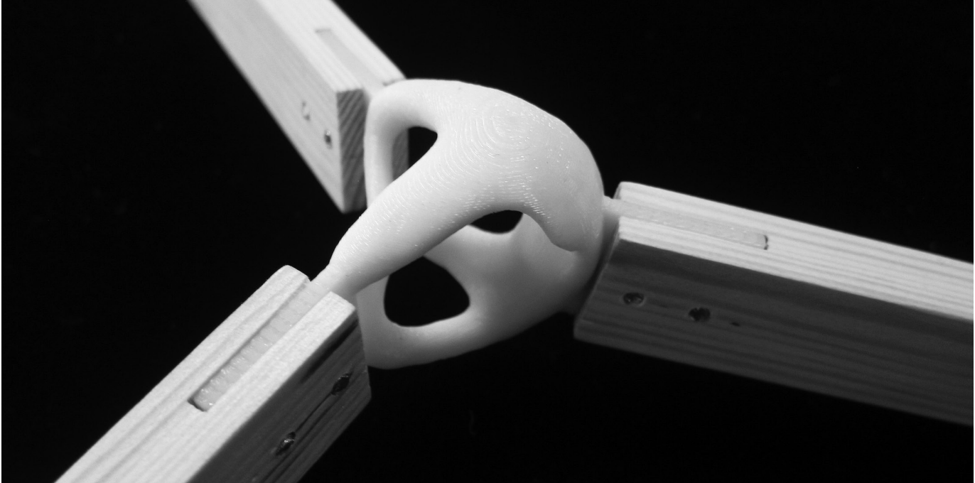
5 Scaled Prototype – FDM print of node resulting from generic load conditions
