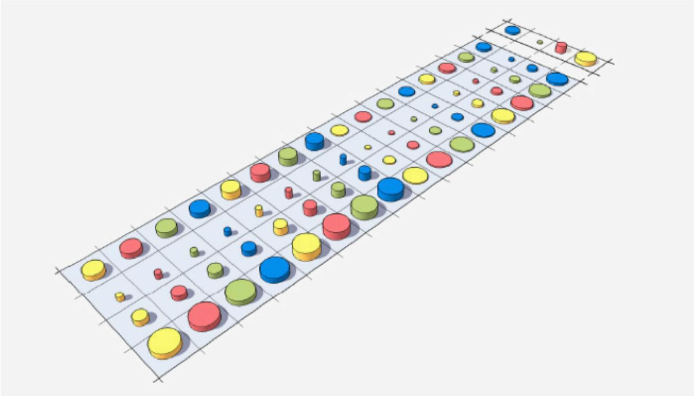
1 A parametric cylinder with four possible heights, radii and color values can create sixty-four alternative solutions
