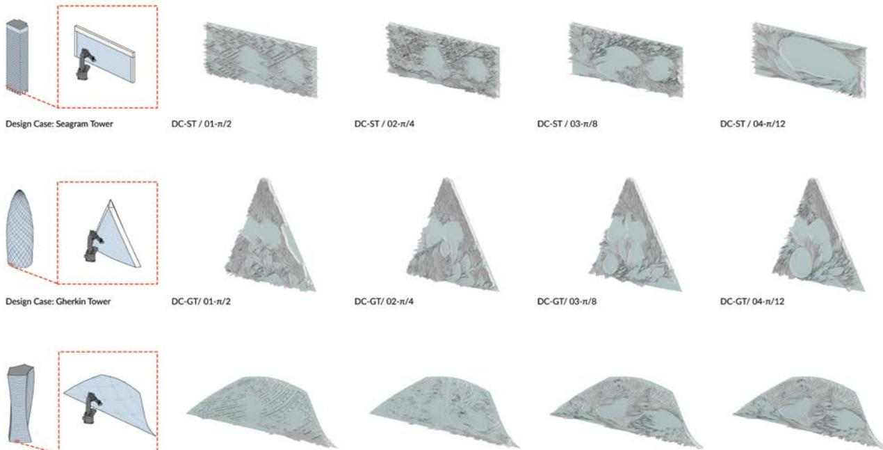
6 Image showing design alternatives for 3 different building case studies, which represent different levels of complexity (flat surface, curvilinear surface, free-form surface).
