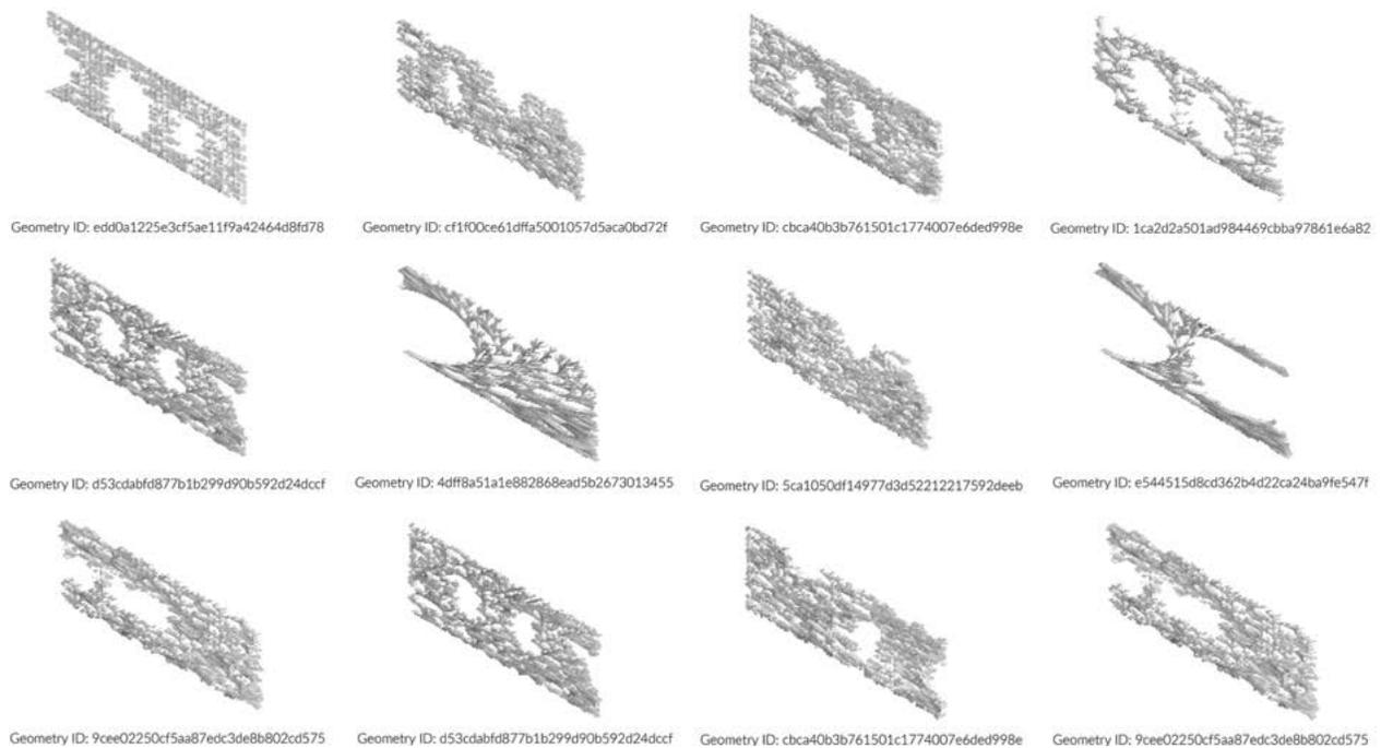
3 A subset of generated facade panel alternatives, with 2 and 3 openings on a planar input surface, which are high ranking in terms of environmental performance and therefore are tested for their constructability.
