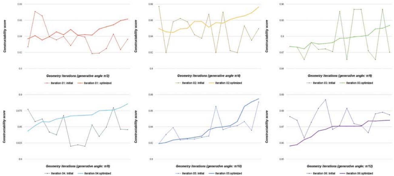
5 The graphs illustrate 6 different design generation cycles with variable angles with (bold, dark lines) and without (thin, light lines) the constructability score improvement over time per geometric iteration.
