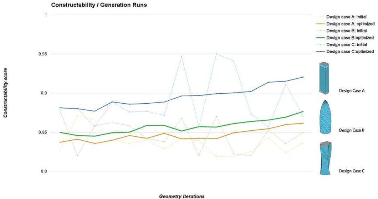
7 Constructability metric in relation to design iterations for each of the different experimental case studies. Light curves represent the non-robotic-agent optimized constructability, bold curves represent the design generation inclusive of the robotic agency optimization.
