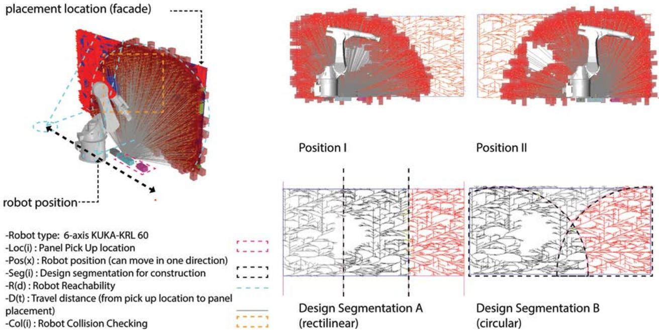
4 Diagram illustrating the design of the experiment for the simulation of the robotic fabrication segmentation, positioning, and reachability, collision parameters of the construction agent.
