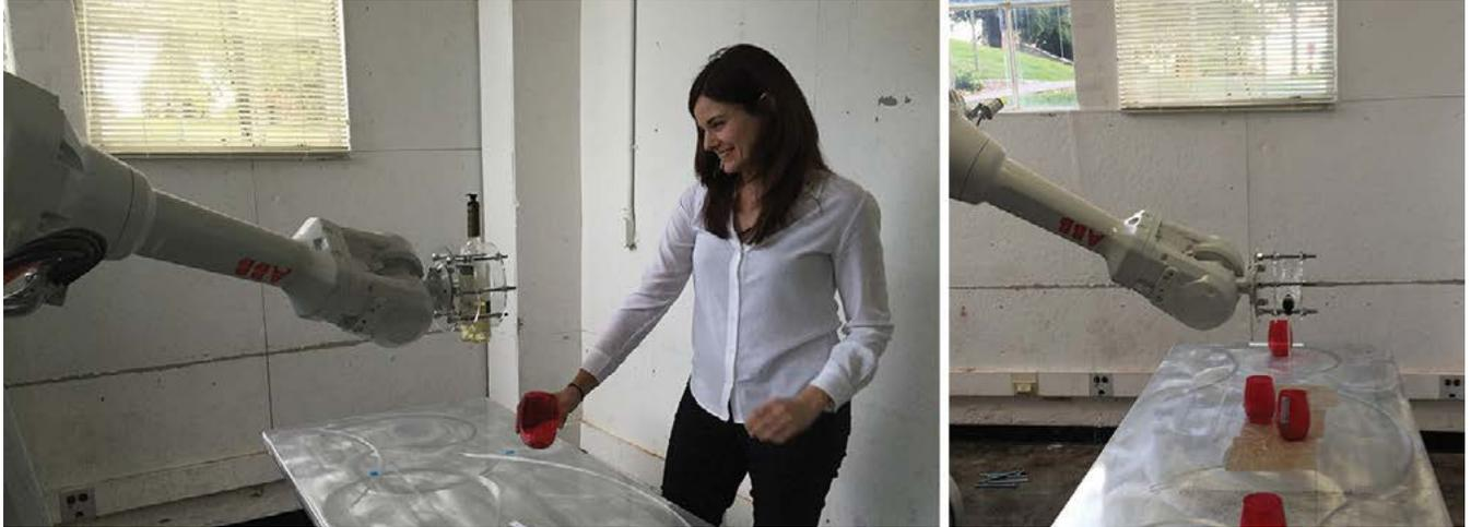
7 Dynamic wine pouring with object detection, shortest path calculation between objects and immediate tool path generation for pouring. This test highlights two levels of feedback: 1. Through a user moving their glass in space and 2. Between multiple glasses in shifting locations on a table. The tool path adjusts accordingly in real time for both cases.
