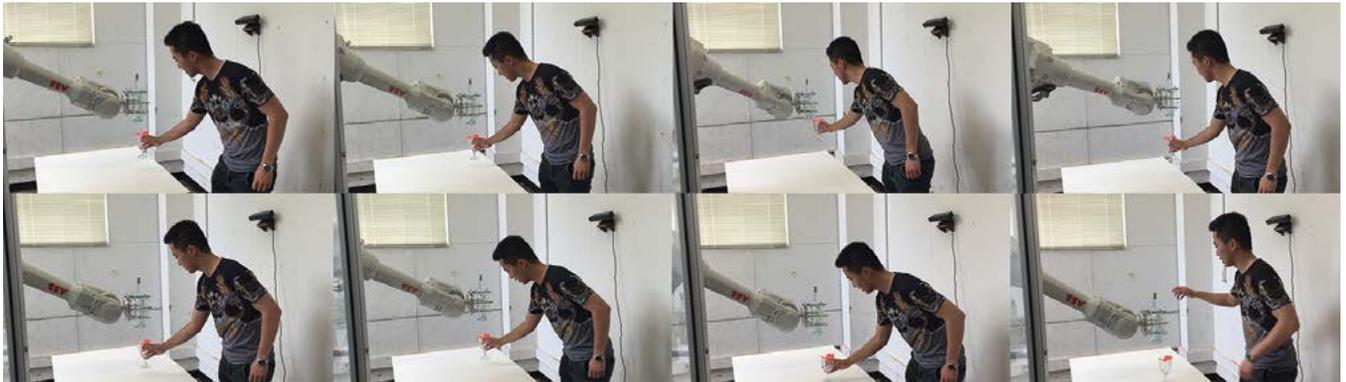
8 Dynamic tracking of glass object in an unpredictable environment for accurate pouring.
