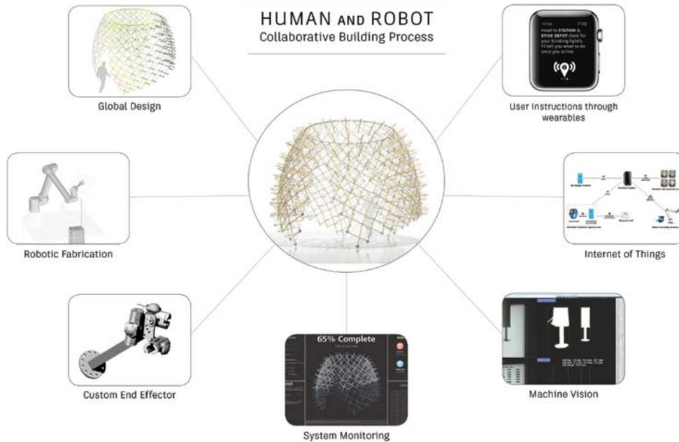
5 System monitoring, connected devices, custom tooling, robotic fabrication, and computational design enabled the development and realization of a human and robot collaborative building process.
