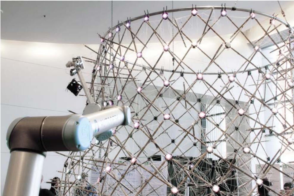
20 Final structure composed out of 224 unique modules fabricated and assembled by human and by robot.
