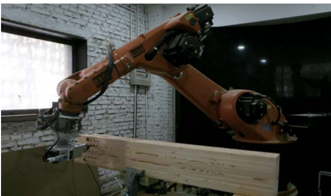
15 Glue Laminating Process of Curved Beam.
