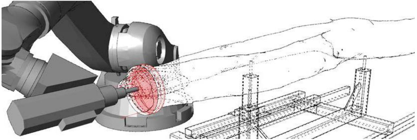
8 Robotic Simulation using in-house algorithms, Kuka-PRC in Grasshopper3d and Rhinoceros3d platform.
