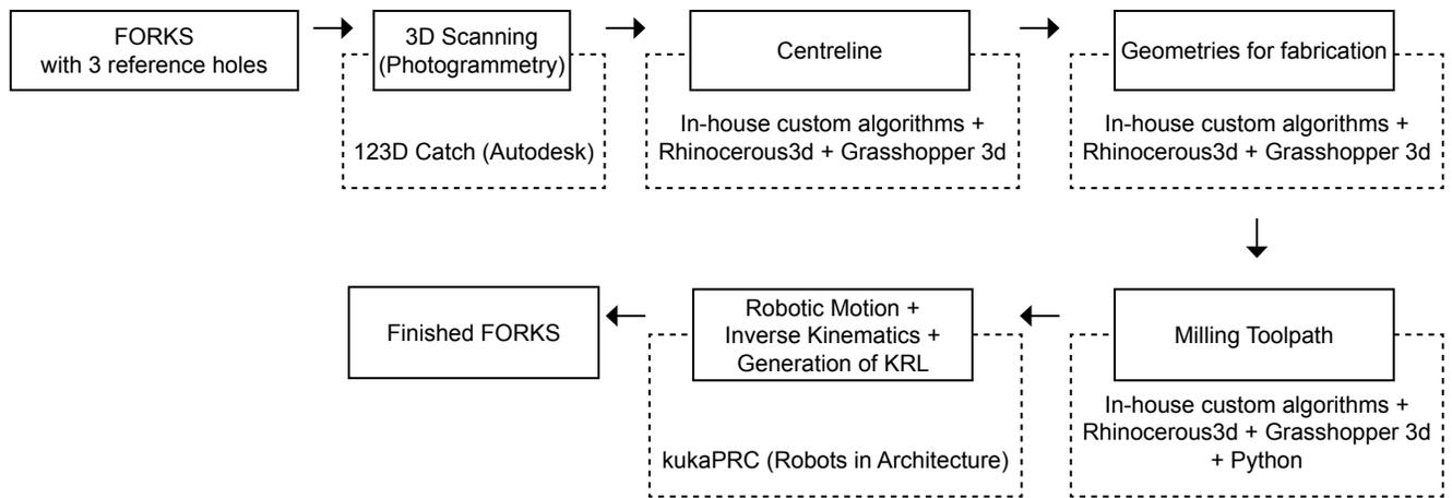
9 Work-flow of the fabrication process.
