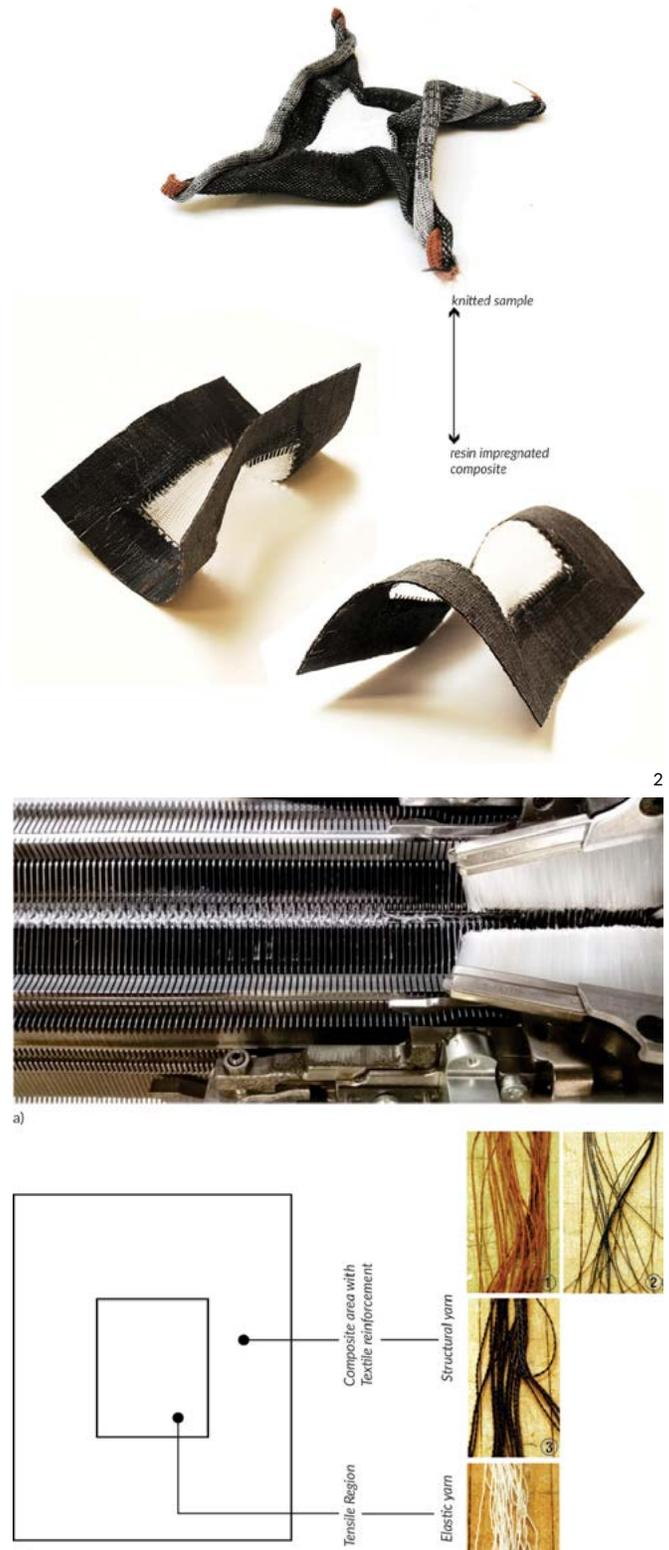
2 Transformation of the knitted sample after the activation of forces through applying prestress and localized composite formation.
