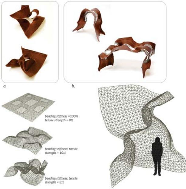
10 Studies showing the possible future trajectories of the research: a) textile hybrid prototypes with multiple reinforcement layers, b) prototypes with shaped and multiple elastic regions, and c) digital model for aggregation of multiple meso-system into one macrosystem.
