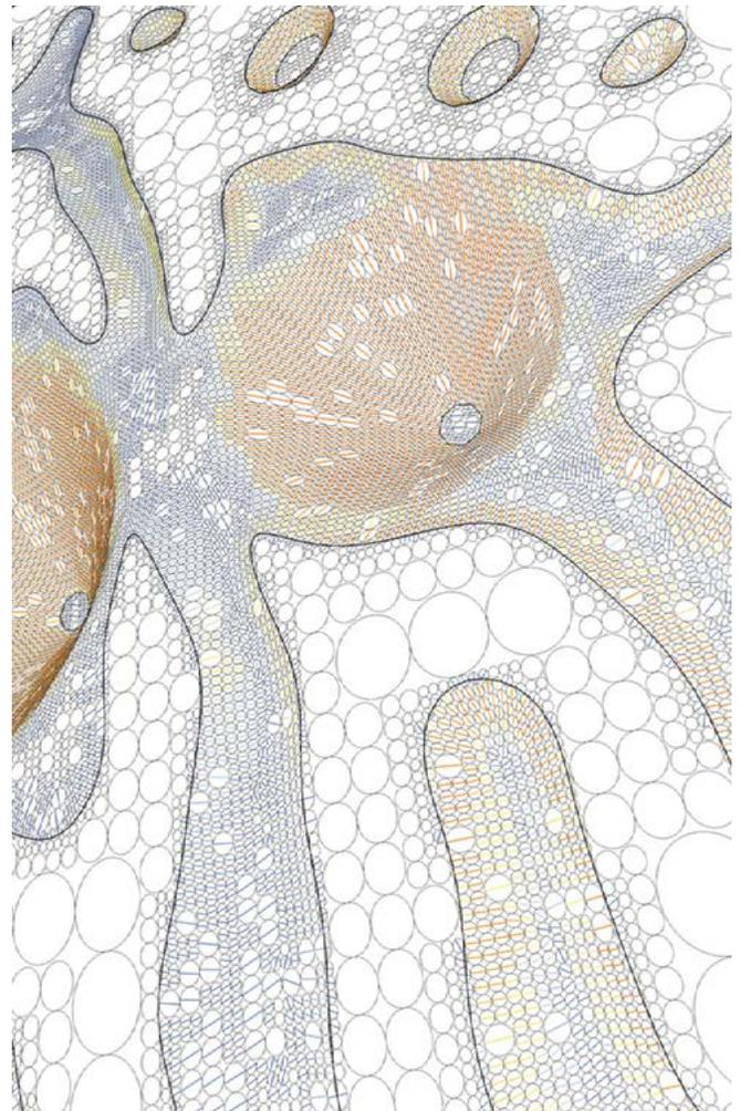
8 Calculation of strains and thinning are achieved using circle projection and a measure of deformation.
