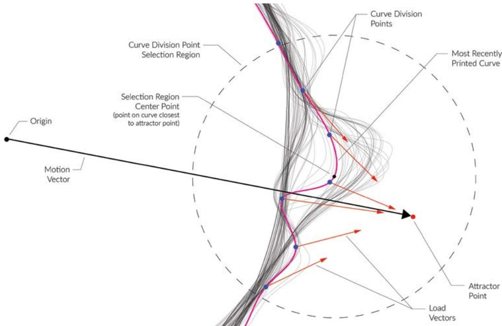
7 Motion vector acting on toolpath. Motion detected by the webcam is translated to a vector emanating from the origin in virtual 3D space, which determines the position of an attractor point. Kangaroo forces pulling on curve division points in the vicinity pull the 3D print toolpath curve toward the attractor point to generate the next layer.
