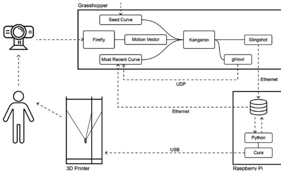
6 Overview of Formeta:3D platform and data flow. Human interaction influences the form produced by the 3D printer, which in turn influences the response of the human. Human and machine are both participants as the machine records the interaction on form.
