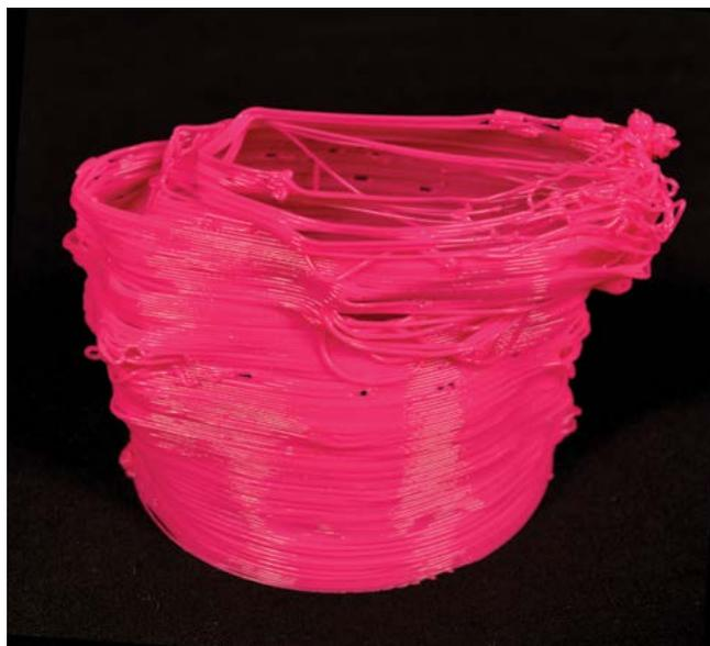
11 3D print resulting from toolpaths shown in Figure 10. The globs of plastic on the top right side are the result of the Kangaroo simulation being overwhelmed by conflicting forces.
