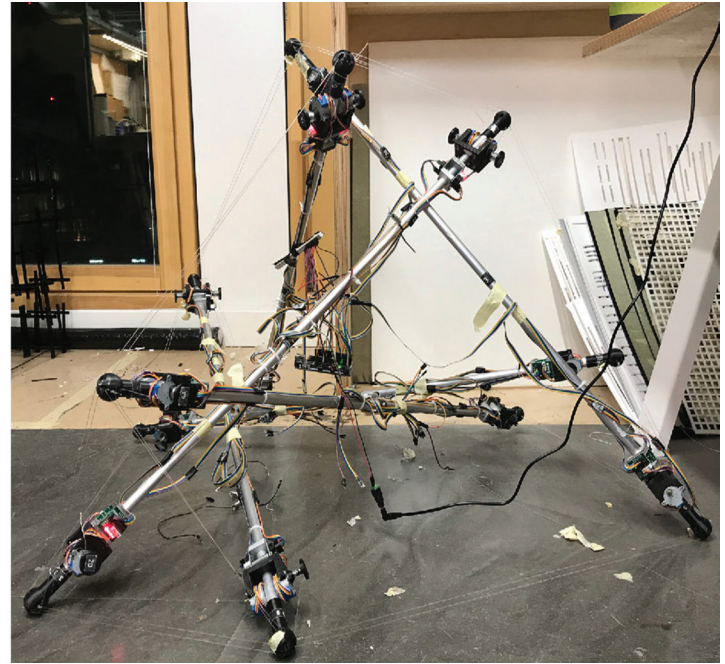
6 -7 Photographs: 1.3m Diameter Tensegrity Robots (Left to Right Icosahedral and Tetrahedral).
