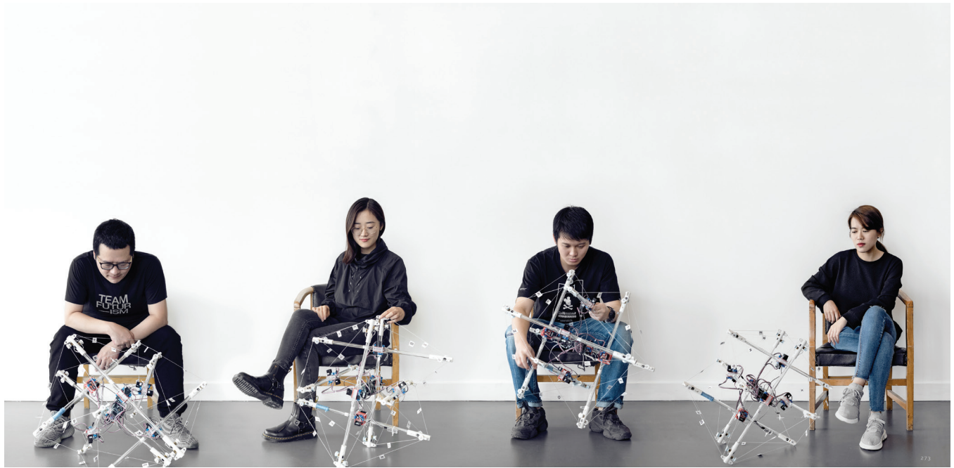
16 Photograph: 600mm Diameter Tensegrity Robot
