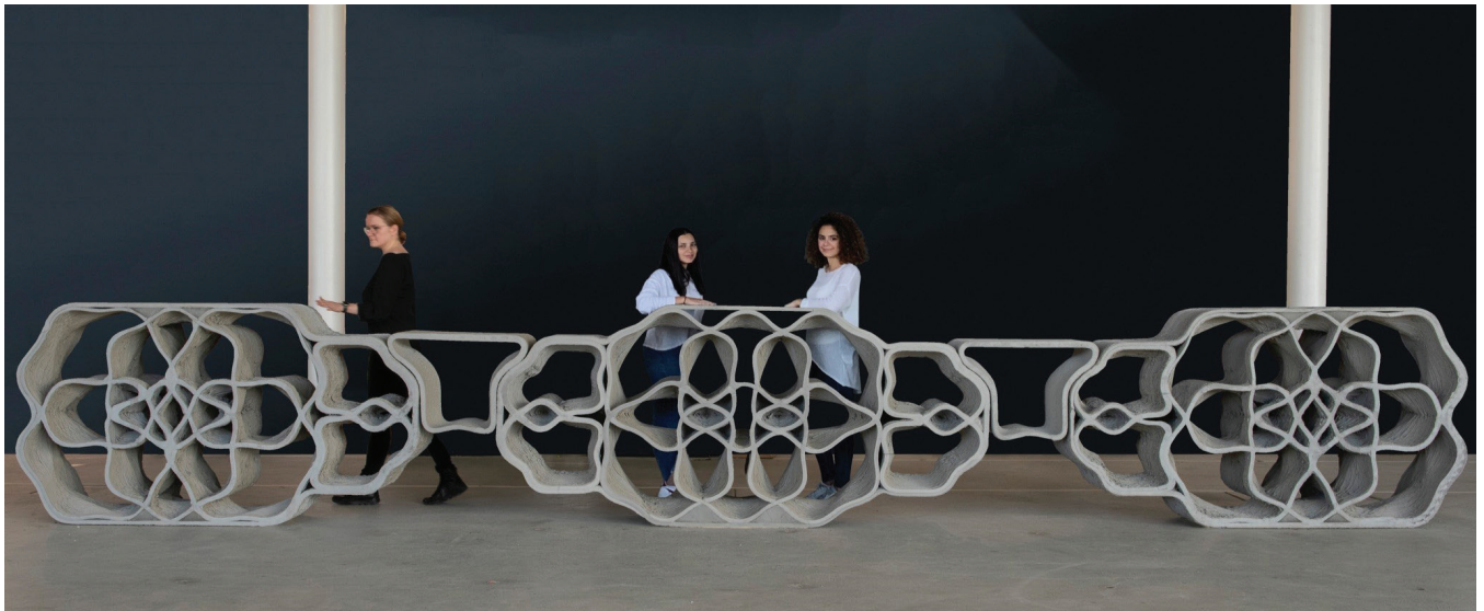
19 Final demonstrator, 3D-printed concrete bar
