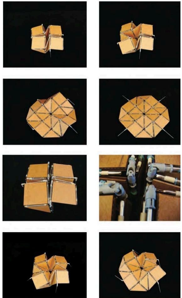
Figure 6. Using a universal joint as a torque converter to allow mechanical movement of the system.
