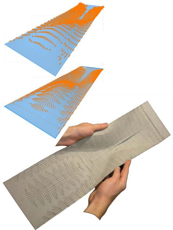
**Figure 6.** Material Analysis, part 3. With a multiplier controlling the various lengths of scores, and the maximum curvature vector providing direction, a rather convincing natural deformation resulted.
