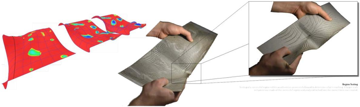
**Figure 5.** Material Analysis, part 2. The surface used for testing the patterning was analyzed for minimum radii curvature. This surface was iterated until the desired minimum curvature was achieved. Then various patterns were tested for natural deformation.
