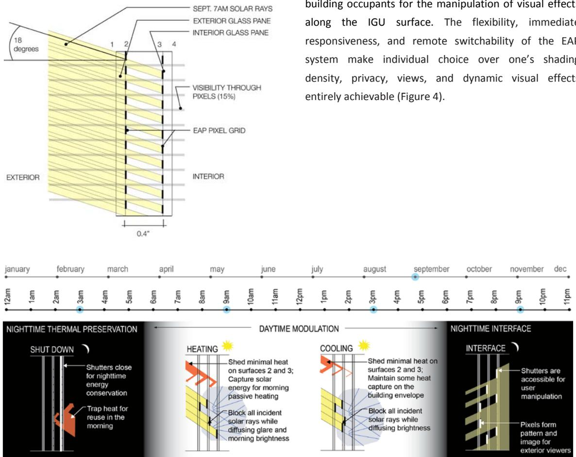
**Figure 4.** Section details of a triple pane electropolymeric glazing design over the course of a September day. Electropolymeric shutters modulate light for diurnal and seasonal variation; at night the façade system can preserve heat, or become an active interface for views
