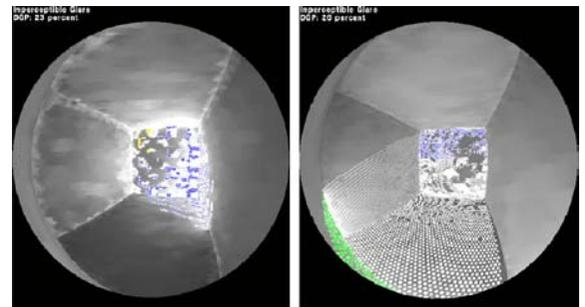
**Figure 9.** Glare probability for a double-layered IGU of both large- and small-scale shutter sizes on a south-facing New York City façade.
