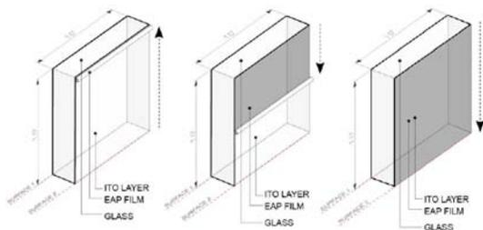
concept for the EAP system is anticipated to outperform comparable technologies due to its effectiveness in modulating solar energy while addressing human desires for daylight, visual comfort and variable optical effects.
