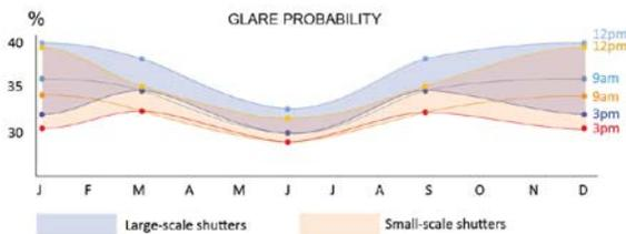
**Figure 8.** Glare probability for large- and small-scale shutter sizes on a south-facing New York City façade indicate that larger shutter sizes could cause more glare over the course of a year.
