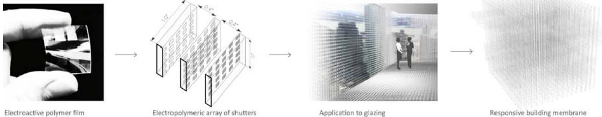
**Figure 1.** Integrating display technology within windows creates environmental modulation and visual diversity along the façade.
