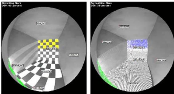
**Figure 7.** Radiance image viewer using the Evalglare tool to identify DGP for large- and small-scale shutter sizes on December 21<sup>st</sup>, 12pm.
