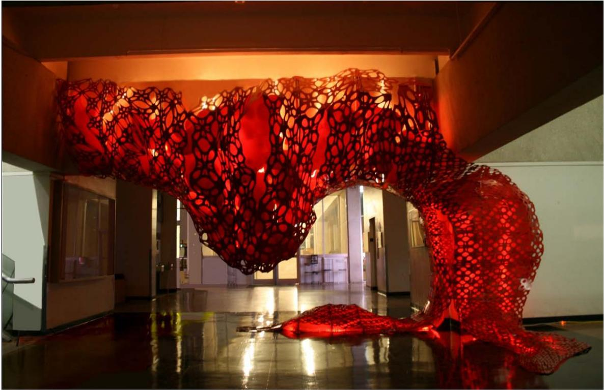
**Figure 1.** The digital fabrication project Swell as built showing two systems: the hard yet porous system (CNC milled surfaces) against a soft interior using laser cutting techniques. Texas A&M University July 2009.
