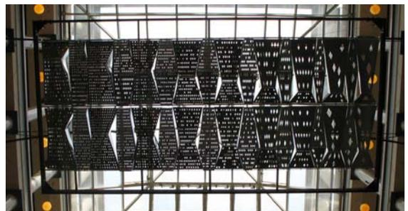
Figure 8. Prototype, full scale. Laser cut aluminum.
