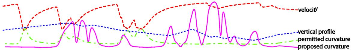
**Figure 12.** Comparison of permitted and proposed vertical curvature.
