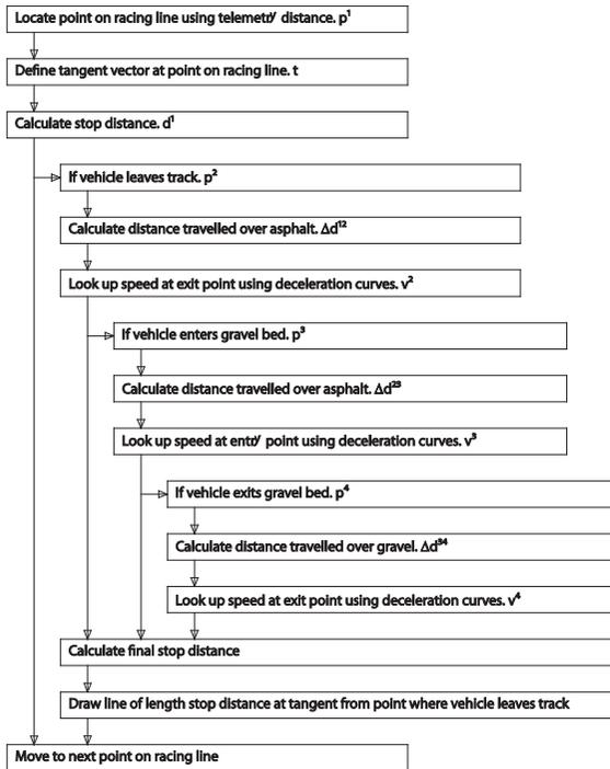
Figure 9. Trajectory generator algorithm.
