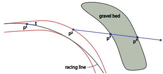
**Figure 8.** Key points for crash trajectory calculation.
