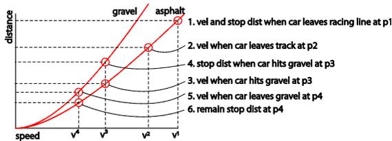
**Figure 7.** Deceleration curves for gravel and asphalt.
