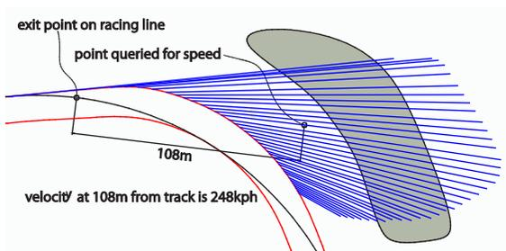
Figure 10. Interrogating a crash trajectory for vehicle velocity at a specific distance from the racing line.
