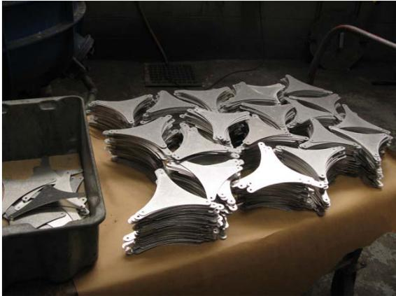
**Figure 5.** 2368 total parts laser cut of 14 gauge aluminum.
