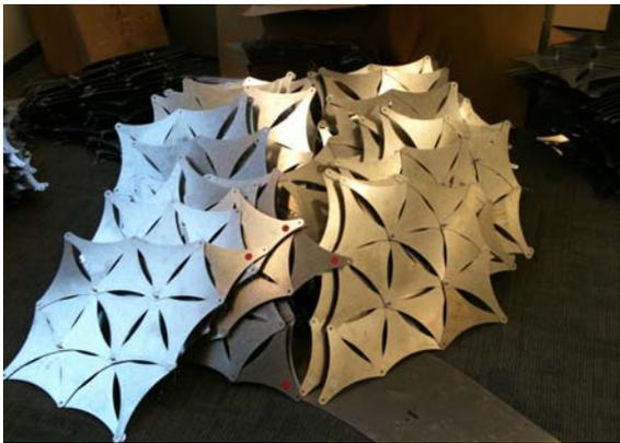
**Figure 6.** Individual pieces assembled into sets of 16 to make 148 quad sections of the Schwarz P Minimal Surface.
