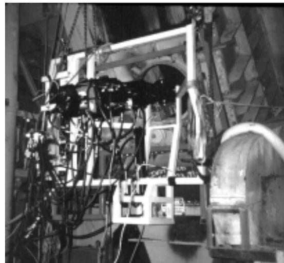
**Fig 8. Clinker Clearing Robot on the Hopper**
