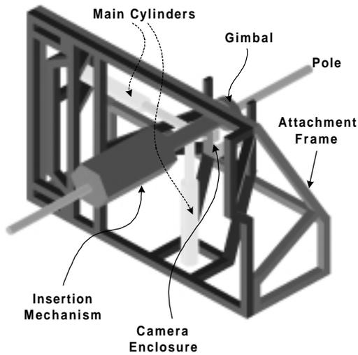
**Fig. 4 Clinker Clearing Robot**
