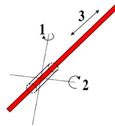
**Fig. 3 Three DOF Spherical Robot**
