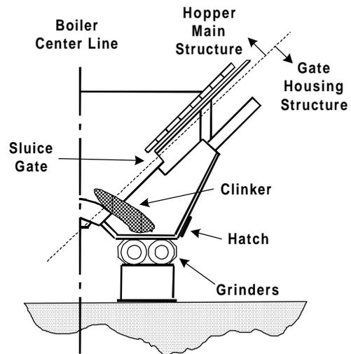
Fig. 1 Half of the Bottom Hopper Structure
