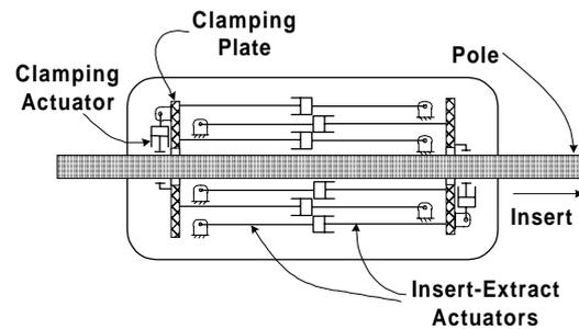
**Fig. 7. A Schematic of the Pole Insertion Mech.**
