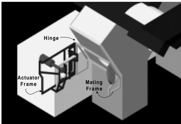
**Fig. 5 Actuator Frame Open for Flushing**
