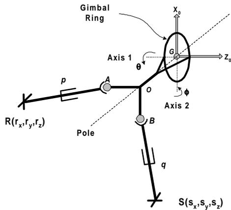
**Fig. 12 Kinematic Structure of the Robot**
