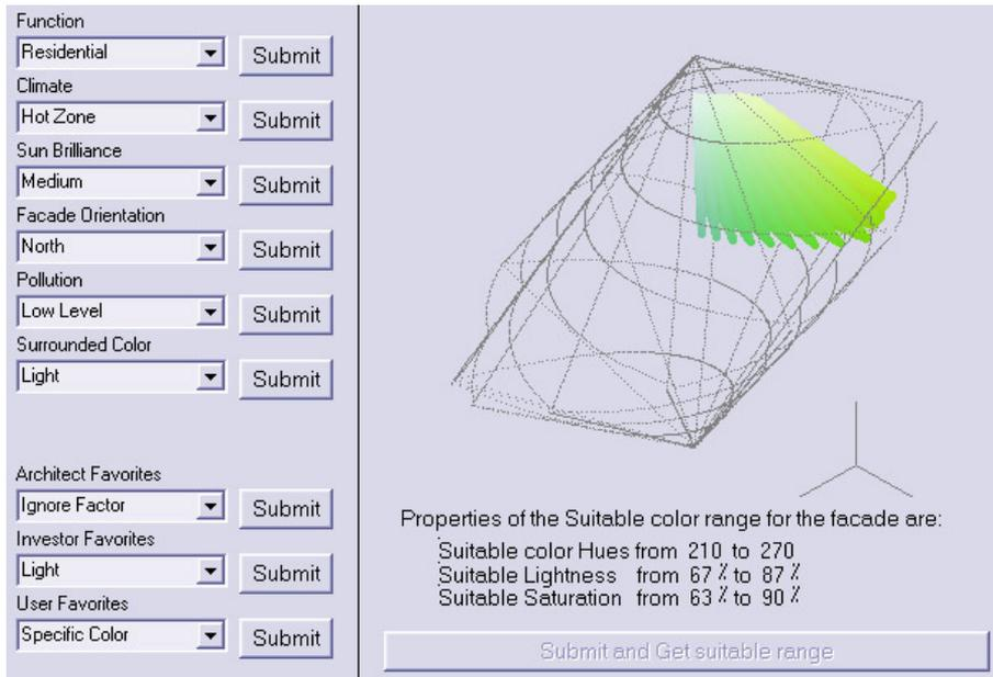
Figure 10. The suitable color range of the facade due to the inserted circumstances and its properties.
