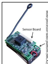
Figure 2. Sensor node with MICA2 and sensor board (photo by the author)
