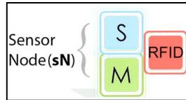
Figure 7. The sensor node design components to be used in this research. “S”: sensor board, “M”: MOTE and RFID tag
