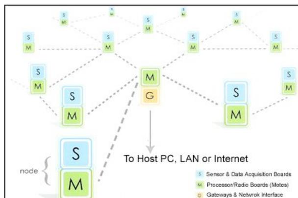
Figure 4. Illustration of the wireless sensor network that forms an ad hoc mesh network. “S”: sensor board, “M”: mote, and “G”: gateway
