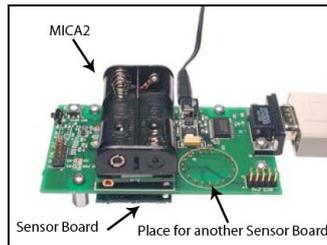
Figure 3. Example of a gateway (MIB510) with MICA2 and sensor board by Crossbow
