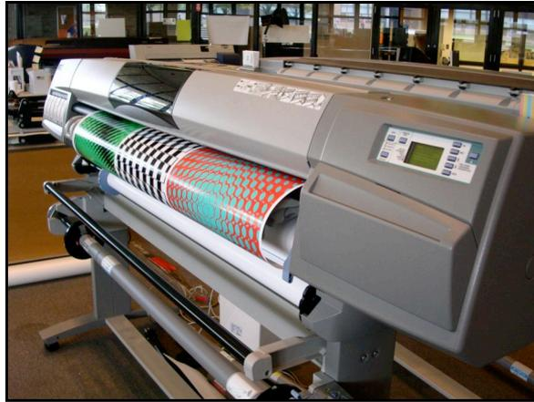
*Figure 4.* The large format inkjet printing machine
