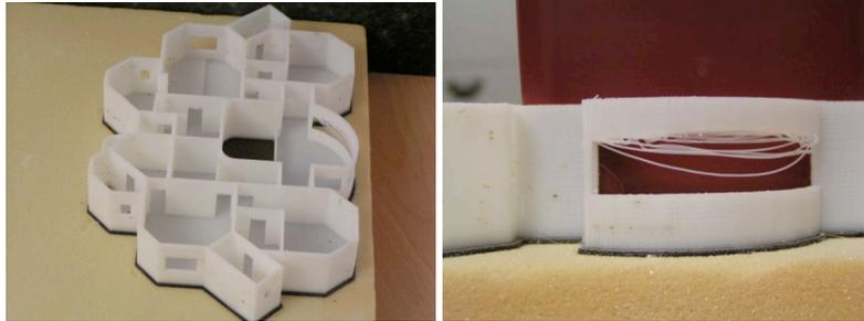
*Figure 10: Errors in FDM RP Prototyping Process*
