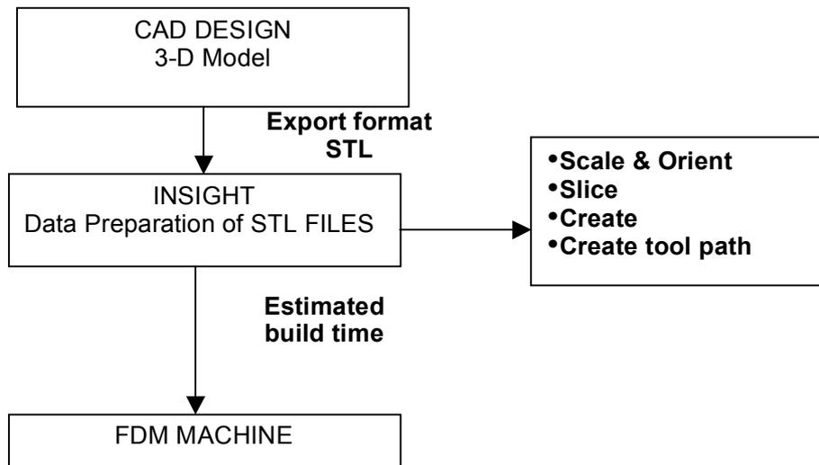
Figure 2: Process flow of RP methodology
