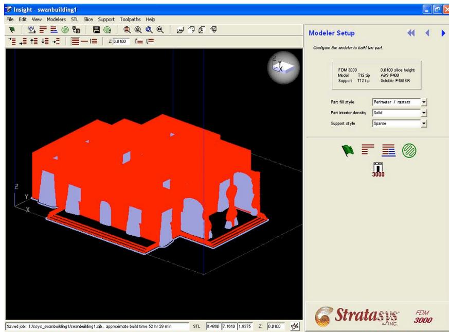
Figure 4: Processing in INSIGHT software showing supports material (blue)
