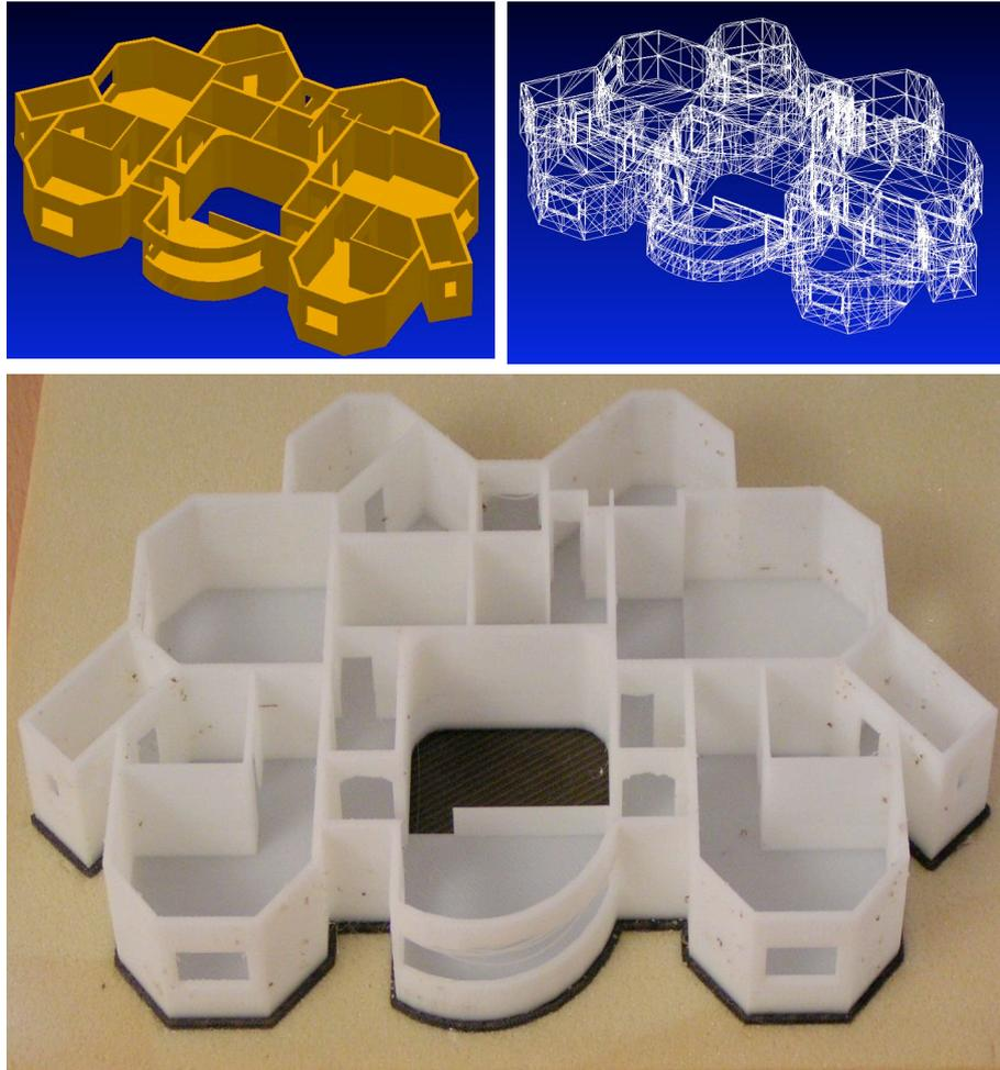
*Figure 6:* Derived from an EDS Ideas 3D CAD Model and manufactured on a FDM Prototype Model created on Stratasys FDM 3000 within hours at The University of Teesside
