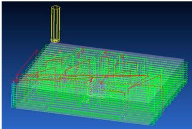
Figure 7: CNC Subtractive Machining: Cutter path simulation of 3D model
