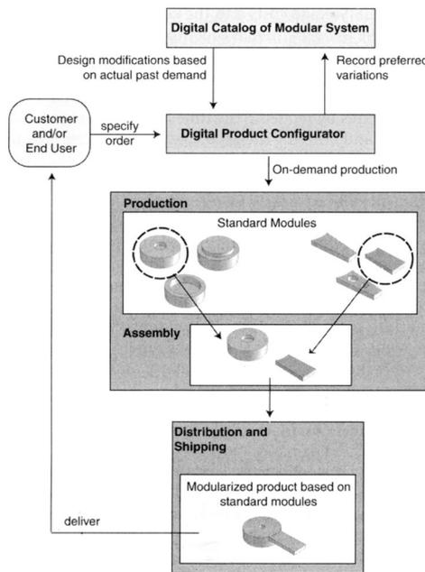
Figure 7. Schematic process diagram of mass customization.
