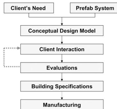
Figure 9. Conceptual Framework of i\_Prefab.
