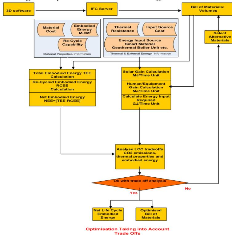
Figure 1. Flow chart for the EIA, LCA and LCCA simulation
