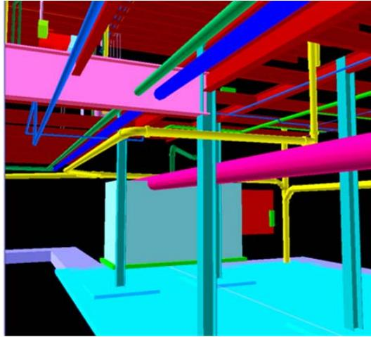
Figure 4 Piping clashing with steel beams at the garage level
