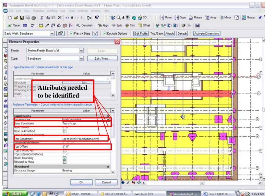
Figure 9. Attributes needed to be identified for a built-in object
