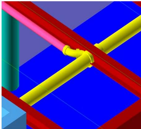
Figure 7. W8 penetrated by an 8" sanitary pipe
