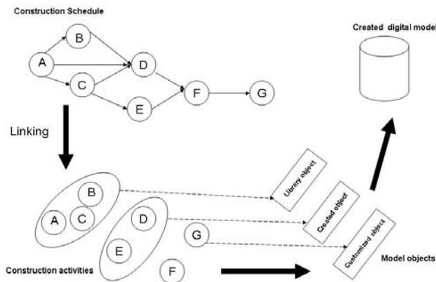
Figure 1 Development process of the digital model
