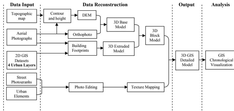
Figure 4. Process Framework for 3D GIS Modeling
