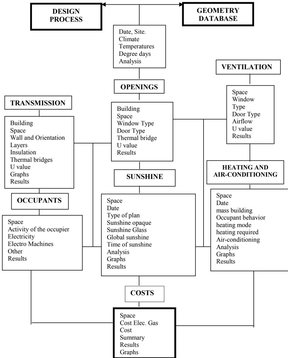
Figure 2, Diagram of SimulArch.
