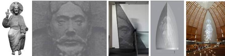
*Figures 24-28.* 24: the original image used for the wall; 25: a portion of the image, rendered with circular perforations of varying size; 26: a mock-up of a single panel (as an indication of its size, note that one of the ceiling panels needed to be removed in order to display it); 27: a model of the wall with the perforated image; 28: a photograph of the wall in the cathedral after completion.
