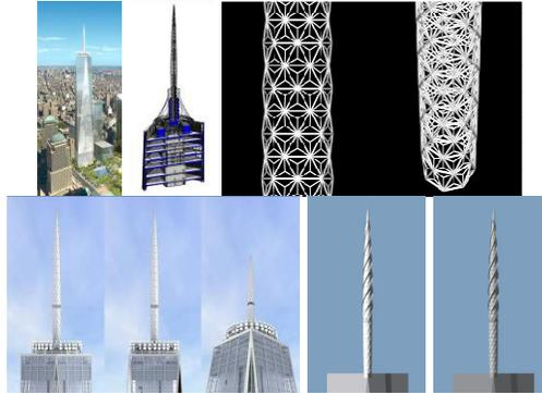
*Figures 34-42.* 34: rendering of World Trade Center Tower One; 35: sectional view of top of building including spire; 36-37: model of one (of many) version of a lattice enclosure for the spire; 38-40: three views of the spire as a fully-enclosed structure; 41-42: renderings of the spire with "helical strakes" for additional wind resistance (showing variation in light and shadow at different times of the day).
