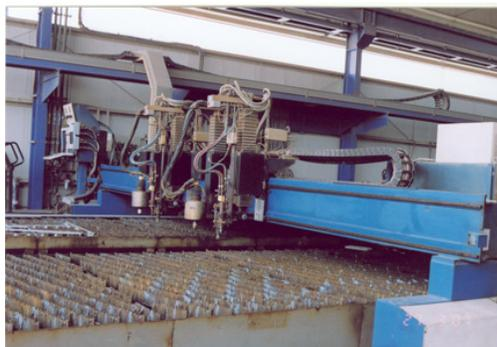
Figure 6. Plasma cutting unit (Abu-Dhabi Ship-Building)
