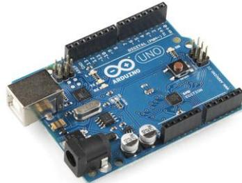
Figure 1. Arduino microcontroller board
