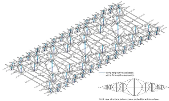
Figure 4. Differential cell size lattice assembly and the actuation logic.
