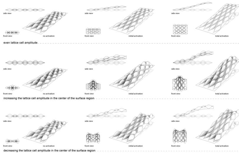
Figure 7. Choreographing the surface movement by changing the lattice cell size/amplitude.
