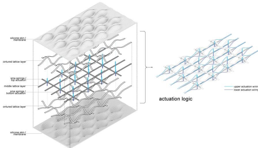
Figure 3. Lattice assembly and the actuation logic.
