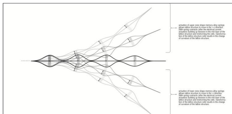
Figure 1. Amplitude of bending and cell deformation after SMA spring actuation.
