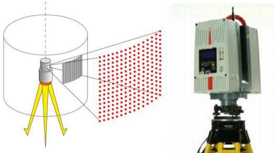
Figure 10. Digitalization technique with a 3D scanner
