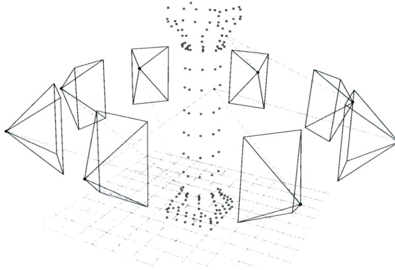
Figure 2. Principle of taking pictures of the architectural object
