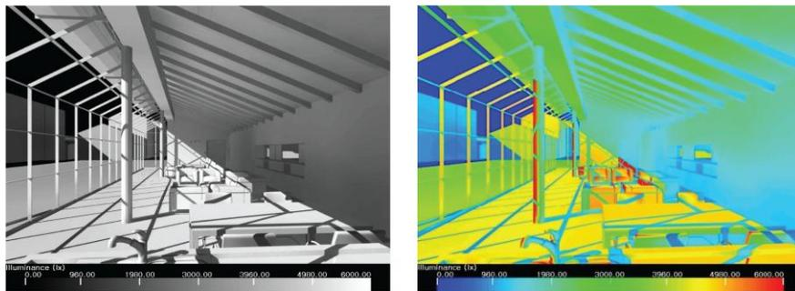
Figure 2. Solar radiation simulation indicating the angle and intensity of the incoming sunlight in the prototype, on June 21, at 1 PM, in Trento, N. Italy
