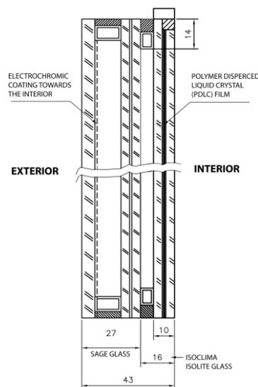
Figure 5. Section of the typical windowpane exposing the layering of materials.
