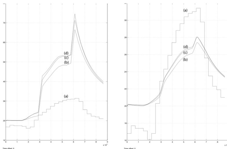
Figure 6. Results of temperature simulation during summer with all the electrochromic panes clear (left) and tinted (right). Curve (a) corresponds to the exterior temperature. Curves (b), (c) and (d) correspond to the interior temperature in the three modules of the prototype.
