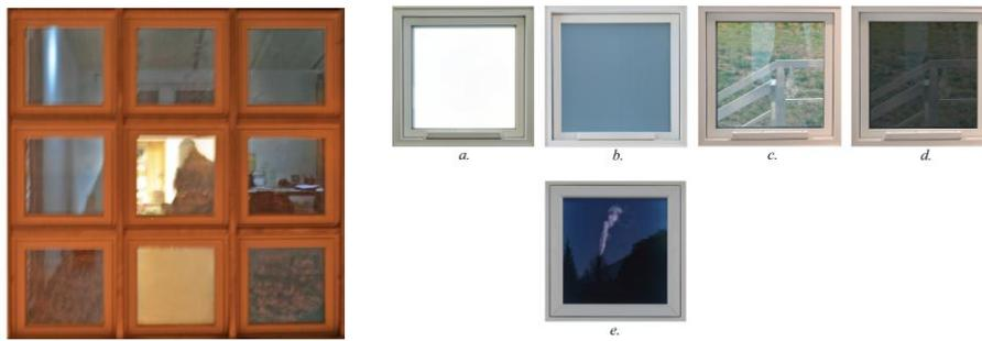
Figure 7. Left: Window pattern involving active electrochromic and PDLC layers. Right: Basic combinations of states. a, b, c, d present window views from the house interior, while e presents a view from the house exterior.
